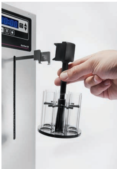
→ Self-centering basket with magnetic coupling
